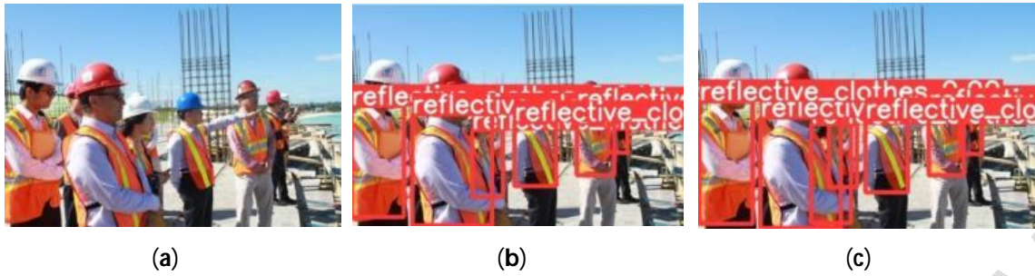
Fig. 12. Comparison of optimization effects of loss functions: (a) The original image; (b) Detection results based on YOLOv3; (c) Detection results of YOLOv3 with DIOU-NMS
