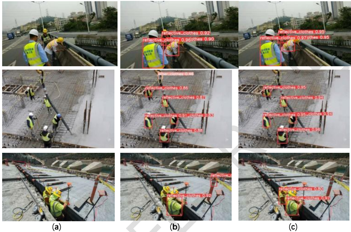
Fig. 11. Comparison of optimization effects of loss functions: (a) The original image; (b) Detection results based on YOLOv3; (c) Detection results of Yolov3 with CIOU-Loss
