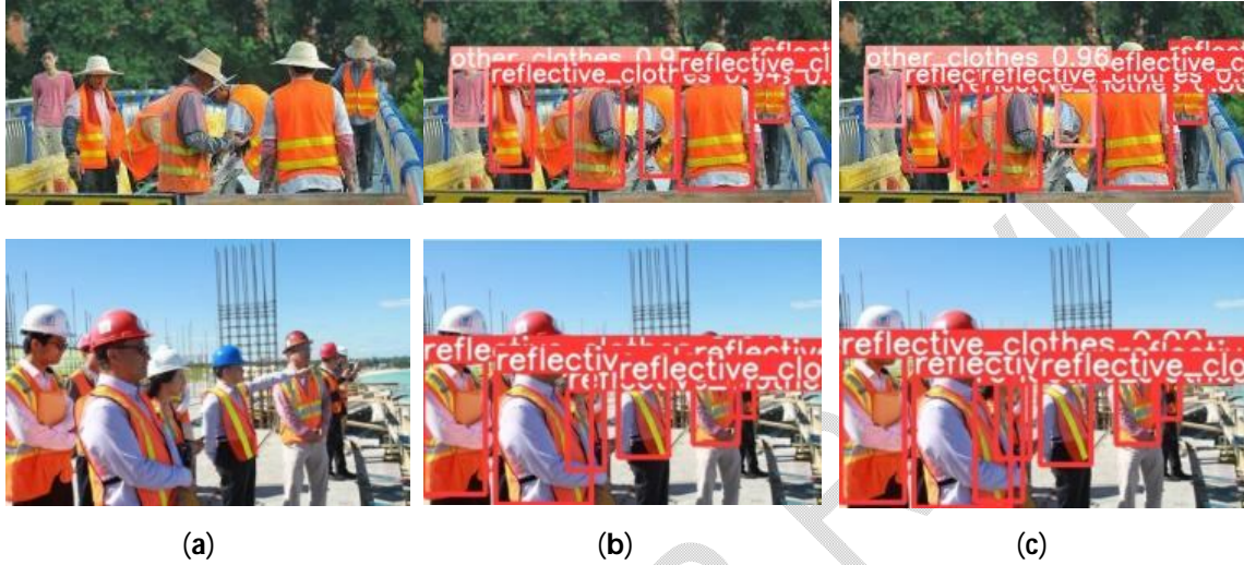
Fig. 12. Comparison of optimization effects of loss functions: (a) The original image; (b) Detection results based on YOLOv3; (c) Detection results of YOLOv3 with DIOU-NMS
