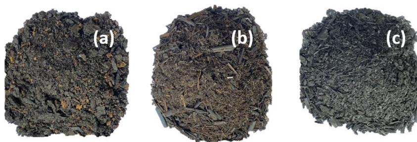
Figure 1. Biochar produced from (a) poultry litter (b) rice straw and (c) pine wood
