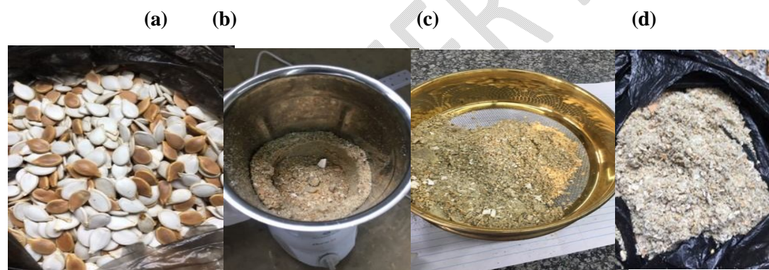
Figure 2 Pumpkin seeds being processed (a) washed to remove b-carotene, (b) blend grinding of seeds (c) retrieving the grounded seeds and (d) powdered feedstock for oil extraction.
