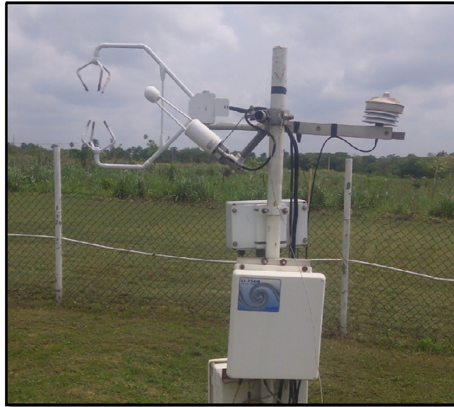
Fig. 2: An Eddy Covariance System Set-up at the Study Site
