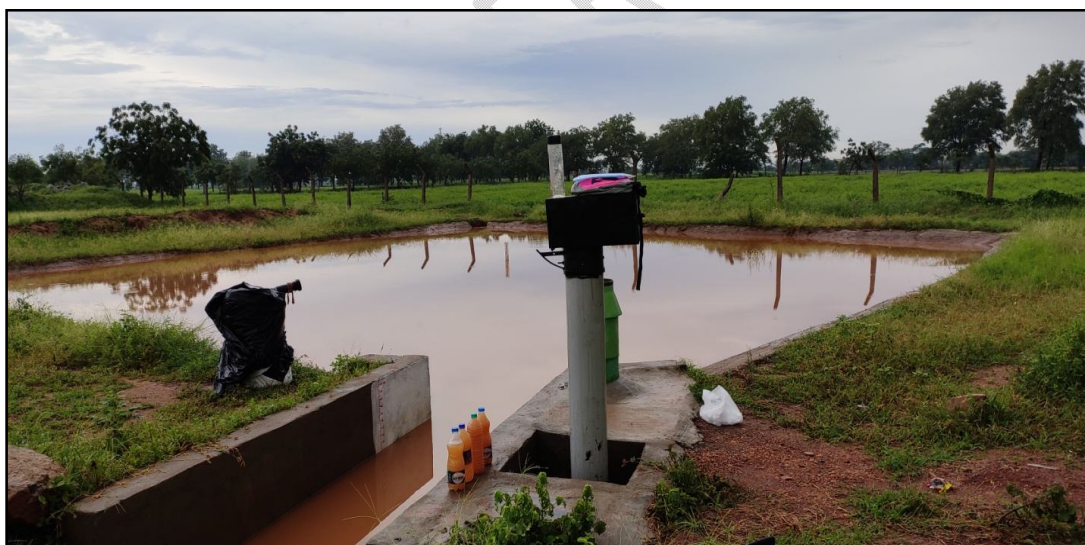
Plate 2b: Image showing the collection of runoff samples from the stilling well for sediment yield calculation
