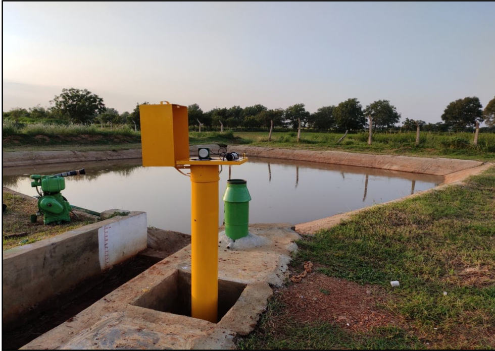
Plate 1a: Image showing setup of Thalimed data encoder, data logger and self recording rain gauge at the inlet section of form pond
