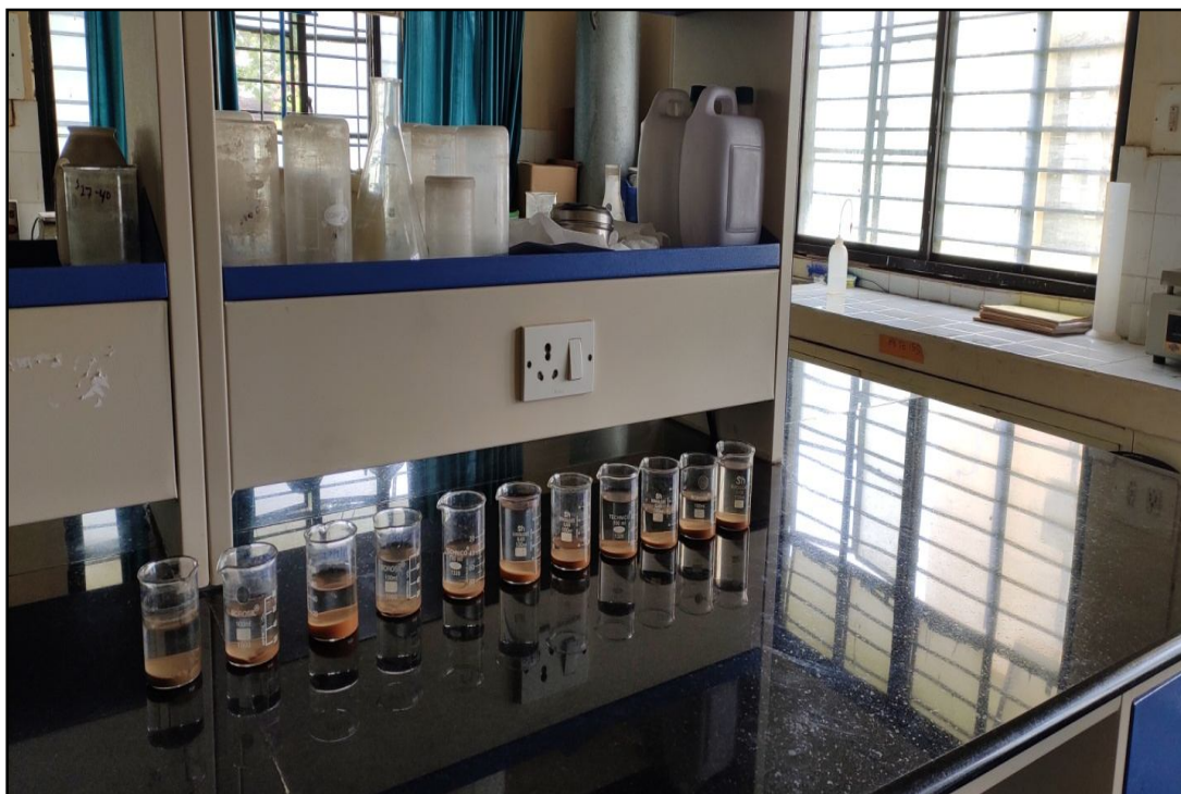
Plate 2a: A view of runoff samples kept for sediment yield measurement in hydrology laboratory
