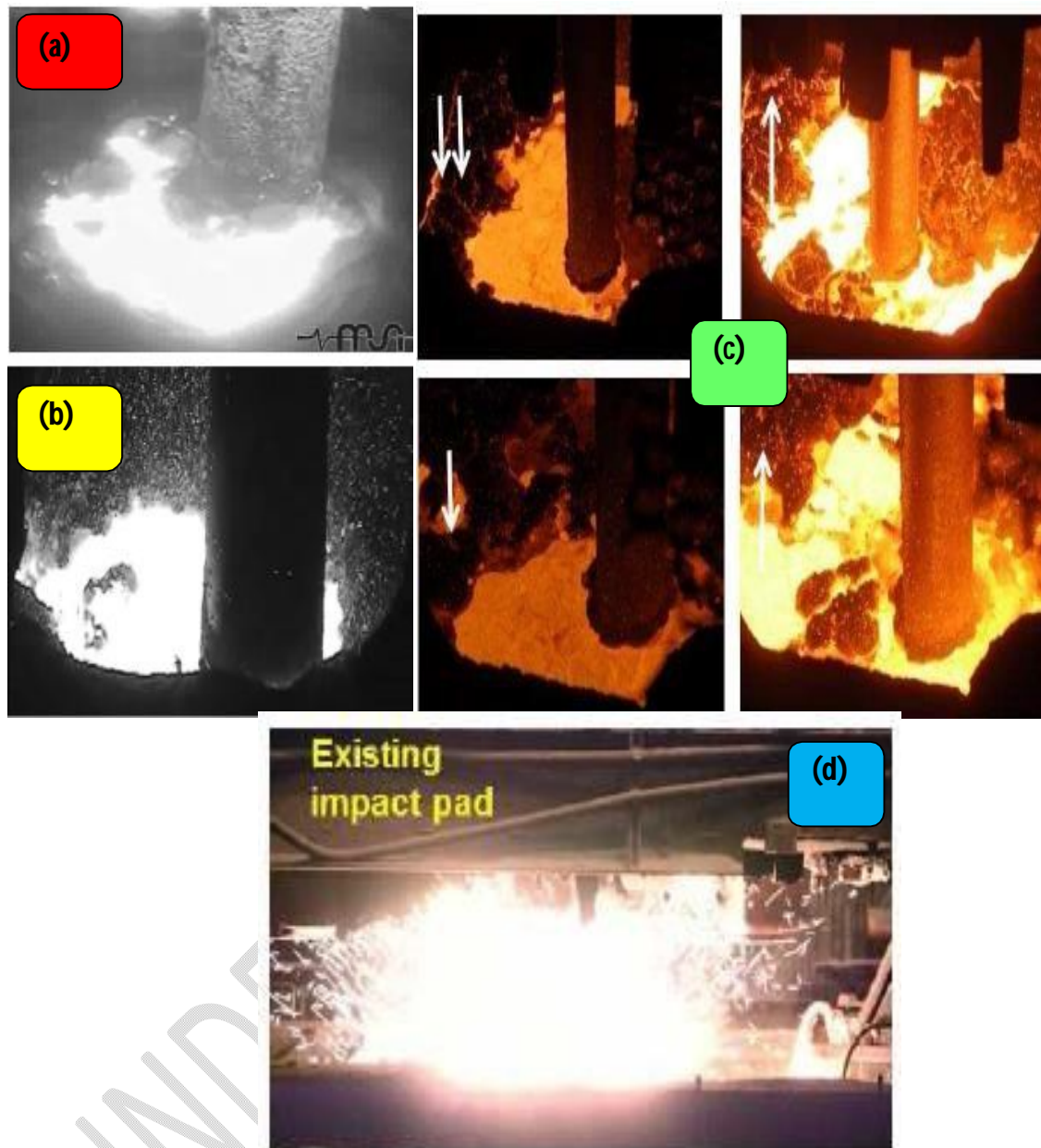
Fig. 2 Industrial observations of slag eye (a), (b) Normal condition(c) Shroud argon purging period and (d) 'Blow Back' effect (Reprinted from [2-3])
