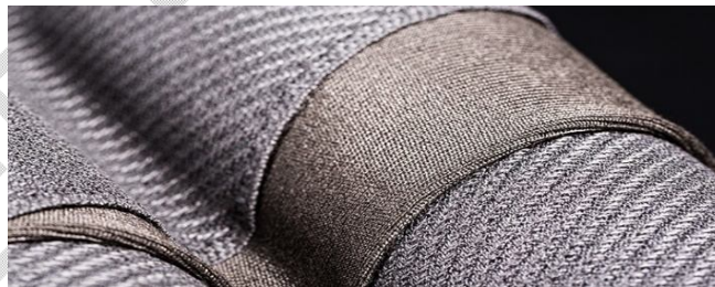
Fig. 5. Integration of metallic threads in the textile
