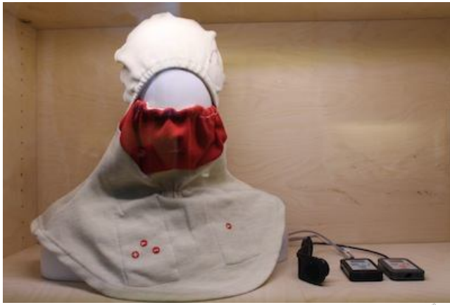
Fig. 15. The smart hood for firefighters [5]
