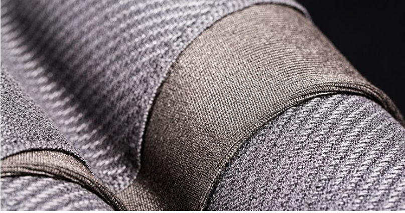
Fig. 5. Integration of metallic threads in the textile
