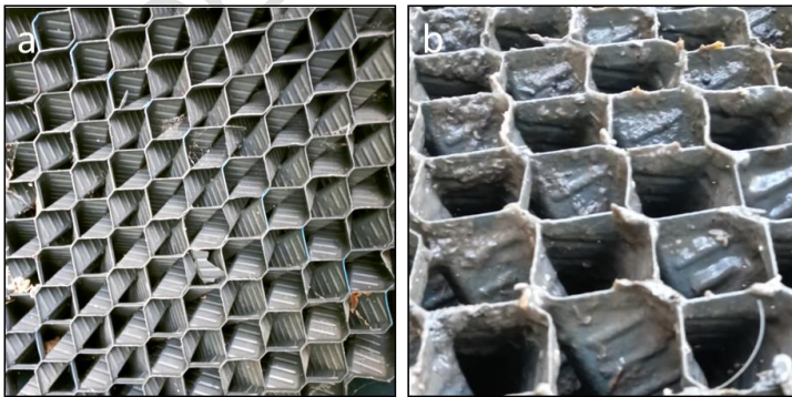
Fig. 9. Bio-tower Growth Media Packaging a) with and b) without biofilm [36]
