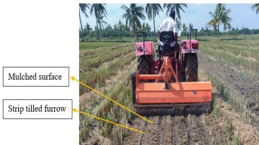
Fig. 5. Mulching cum strip tillage operation by stubble managing unit of the proposed machine
