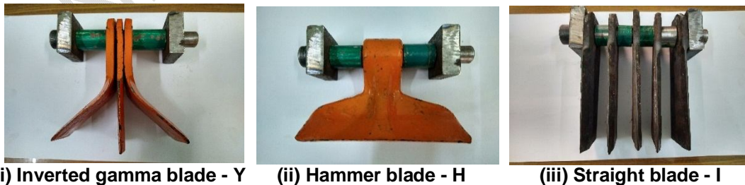
Fig. 2. Type of flail blades selected for the optimization
