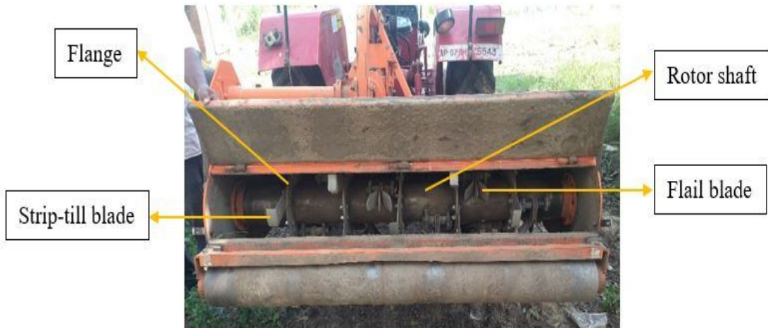
Fig. 4. Mounting of flail and strip-till blades on rotor shaft of stubble managing unit of the proposed machine
