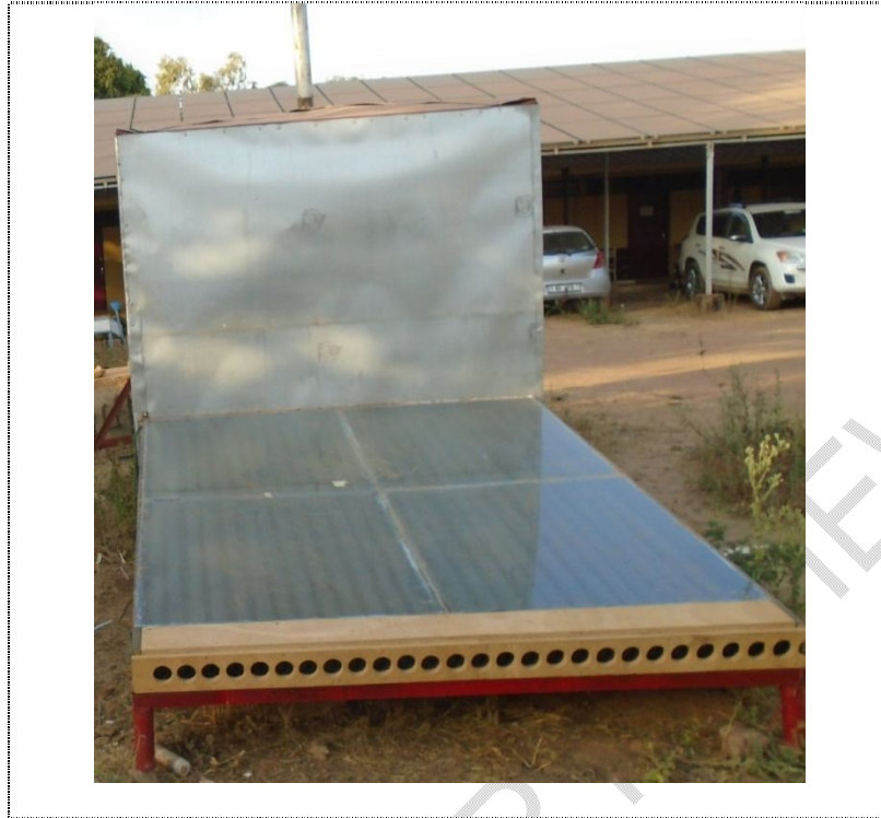
Fig. 3: Solar collector connected to the drying chamber
