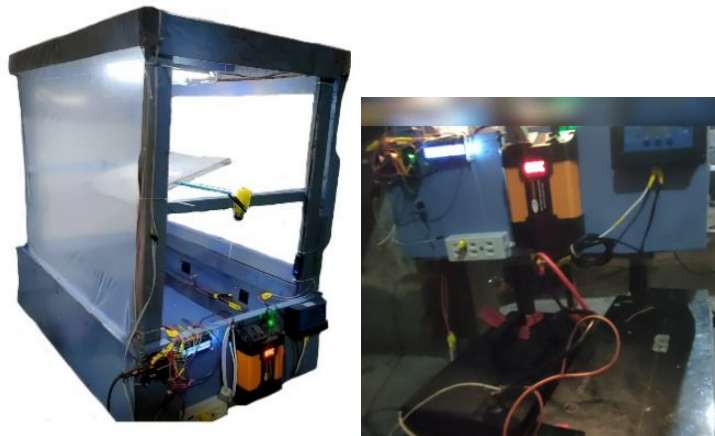
Fig. 14. Automated Squid Dryer Chamber
