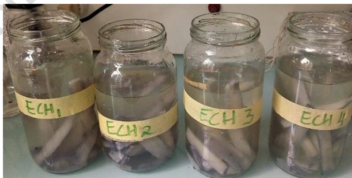
Fig. 4. Chechim nchabe soaking operation in the laboratory
