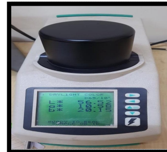
Fig. 2: Hunter Lab Colorimeter
