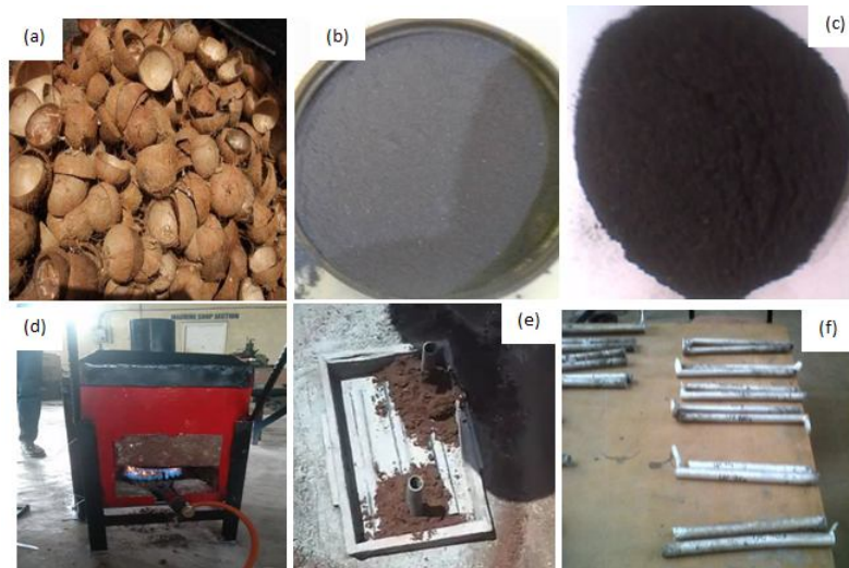
Figure 1: Preparation of samples: (a) Coconut shells (b) Silicon carbide (c) CCS (d) Furnace (e) Molding process (f) Cast samples
