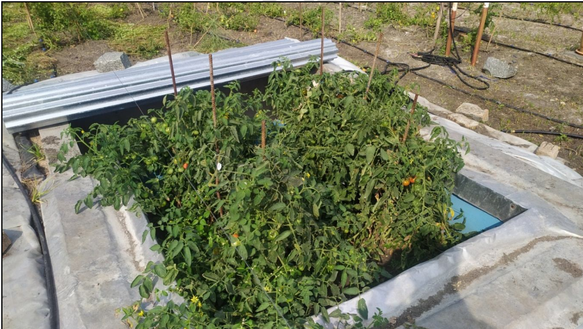
Plate 1. The overall view of the weighing lysimeter with tomato crop
