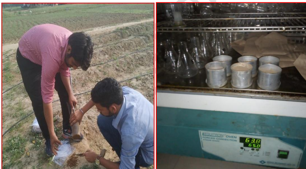
125 126 Fig.2 Collecting soil sample and its analysis for measurement of bulk density and moisture 127 content of soil
