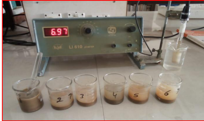
137 138 Fig. 3 Measurement of electrical conductivity of soil samples
