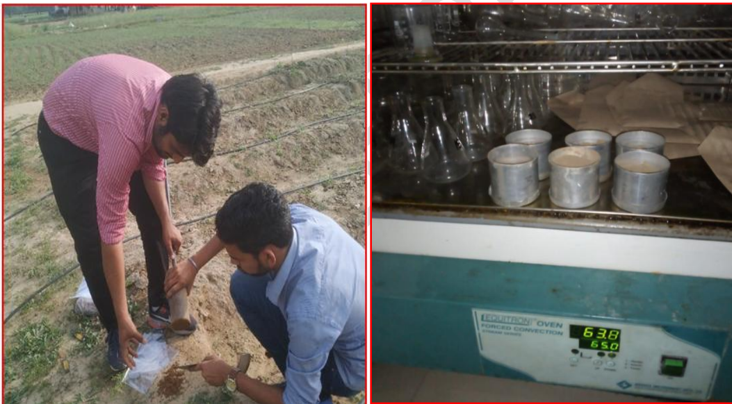
Fig. 2 Collecting soil sample and its analysis for measurement of bulk density and moisture content of soil
