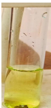
Mixture of solutions of Cl - , Br - , I - , CO 3 2- , NO 3 - , SO 4 2- Ions Figure 8: Effect of selectivity on the colorimetric sensing of I - ions by PCAFC-Cu(II)
