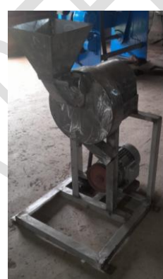
Fig 2: Picture of the Coupled Hammer Mill Machine
