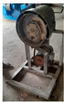
Fig 3: Picture of the Uncoupled Hammer Mill Machine to show the grinding chamber (hammer mills and compartment)
