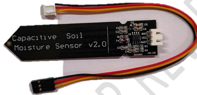
Fig.3. Soil moisture sensors
