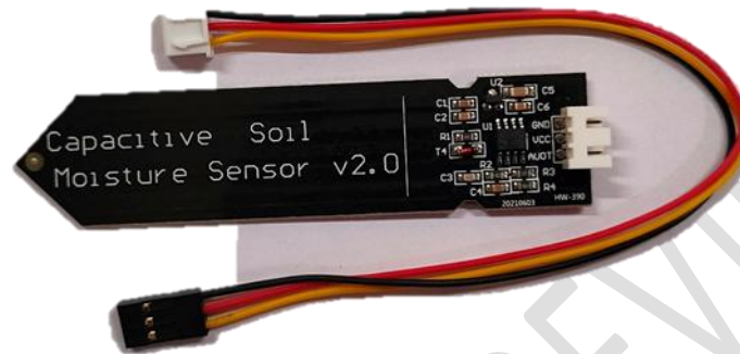
Fig.3. Soil moisture sensors
