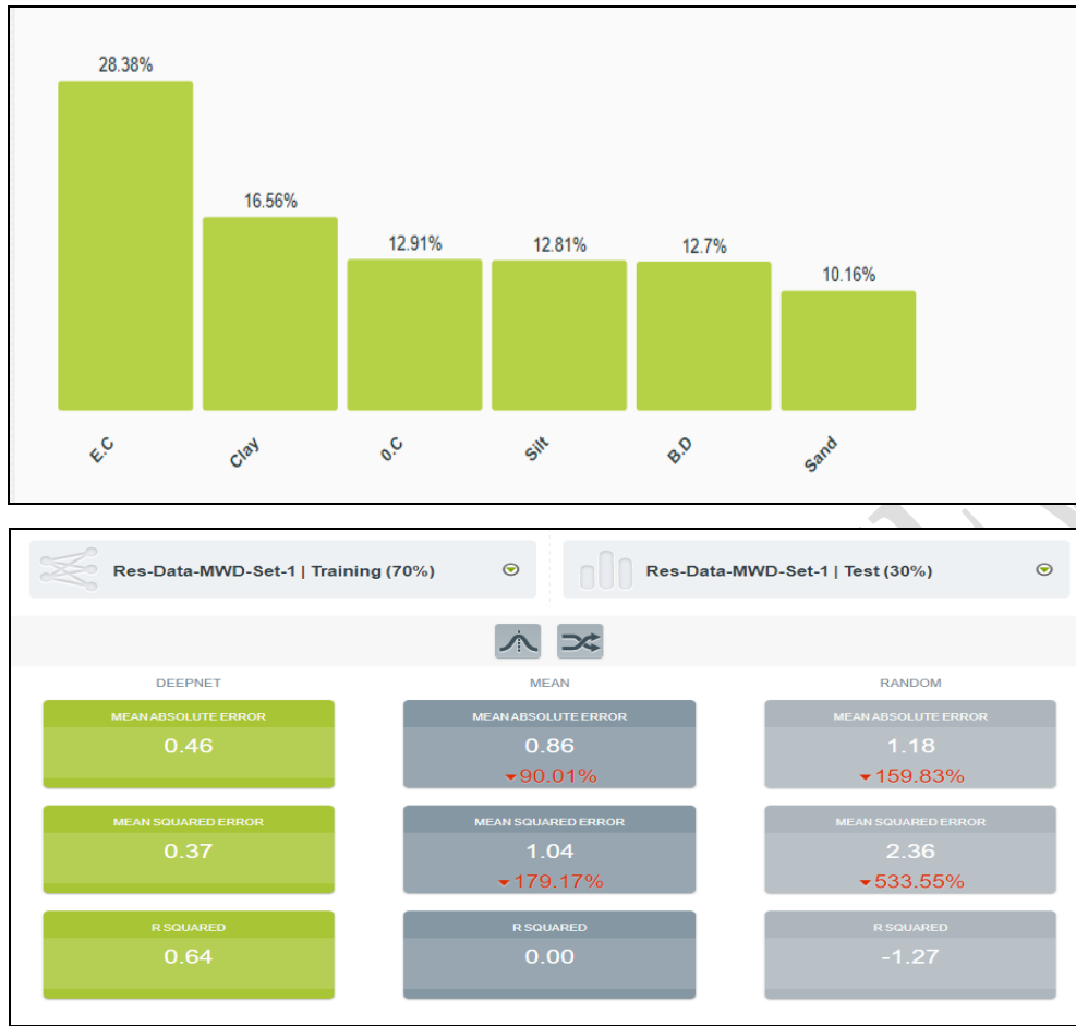
Figure 3. Properties of field importance and Different Regression metrics for MWD using Dataset 1
