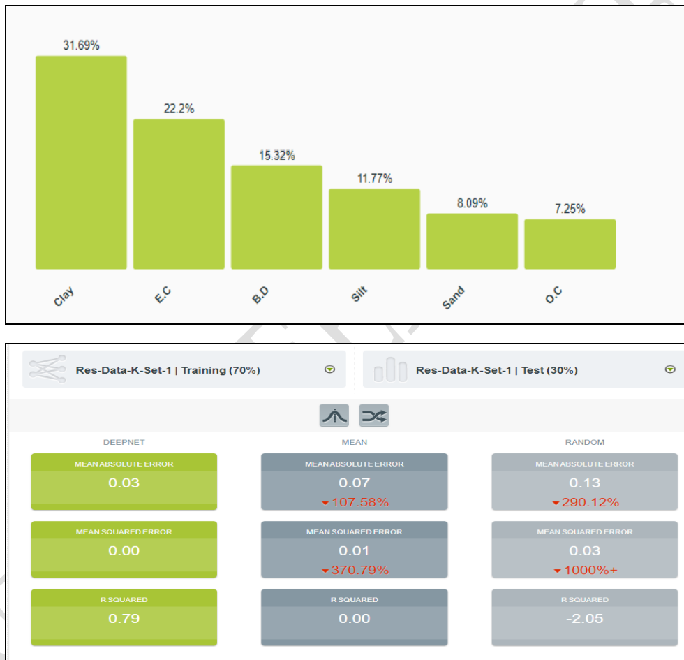
Figure 6. Properties of field importance and Different Regression metrics for K using dataset 1
