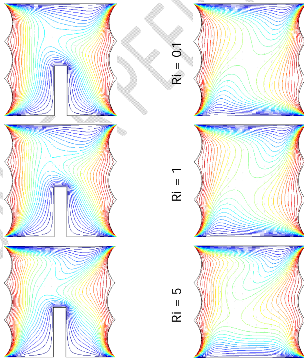
Figure 3: Streamlines with fin for Richardson number Ri = 0.1, 1, 5, 10 while Ha = 50 and Pr = 0.71 .
