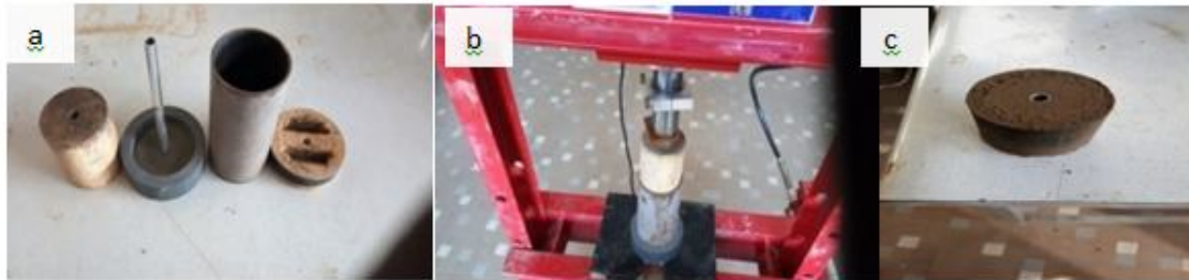
Fig. 2. (a-mold and accessories, b-press for manufacturing specimens; c - manufactured specimen).
