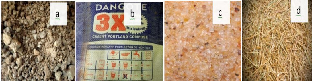
Fig. 1. (a-Clay; b-CPJ 42.5R cement; c- gum arabic; d- rice straw)
