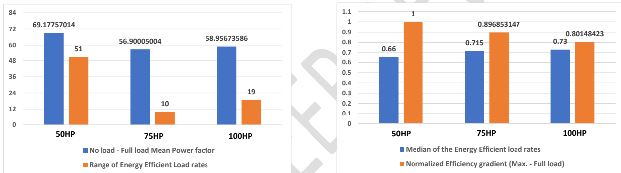
Fig 6: Influence of Power factor and Efficiency on load rates.
