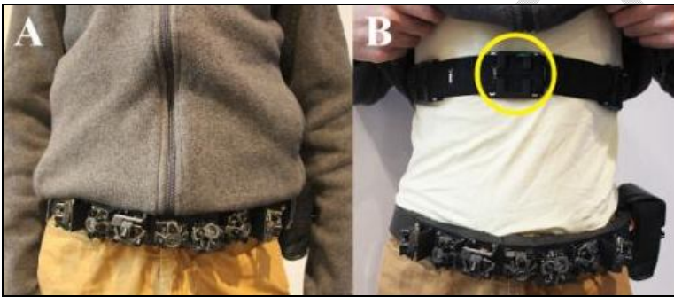
Fig. 4. The ALVU, a wearable device for the visually impaired [13].
