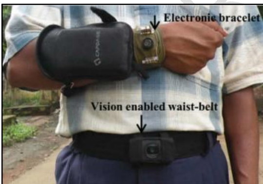
Fig. 6. A blind volunteer showing a typical posture for the use of the electronic bracelet and the vision-activated belt system (EBVEWB) [14].
