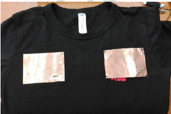
Fig. 7. Proposed portable and contactless ECG T-shirt
