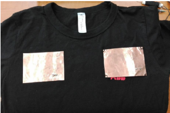
Fig. 7. Proposed portable and contactless ECG T-shirt
