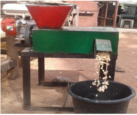
Fig. 5: Cowpea decorticator in operation
