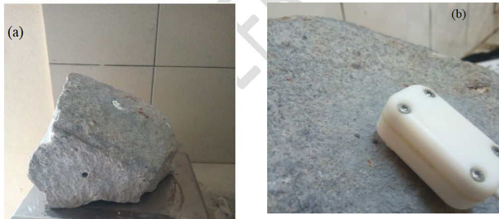
Fig. 2: Thermal conductivity measurement steps: (a) Hole made in the rock, (b) Probe inserted into the hole
