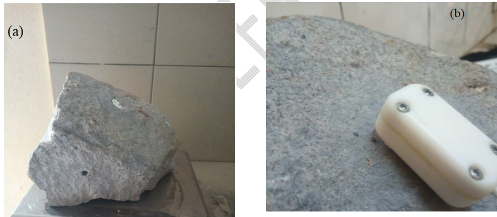
Fig. 2: Thermal conductivity measurement steps: (a) Hole made in the rock, (b) Probe inserted into the hole
