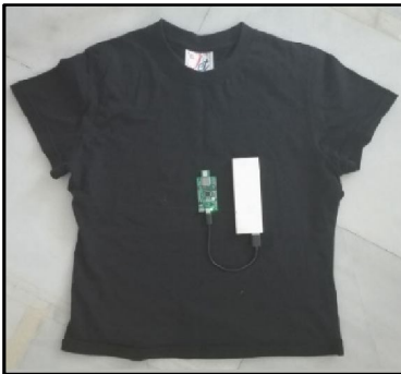
Fig. 10. the experiment T-shirt. The 'Localino' and the power Bank inserted in the clothing of the experiment (A basic cotton t-shirt)
