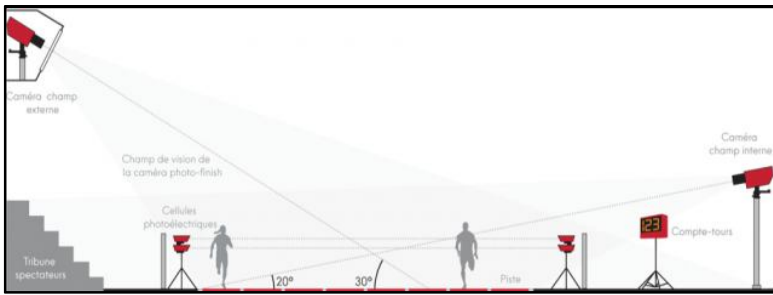
Fig. 3. installation of timing equipment [13]
