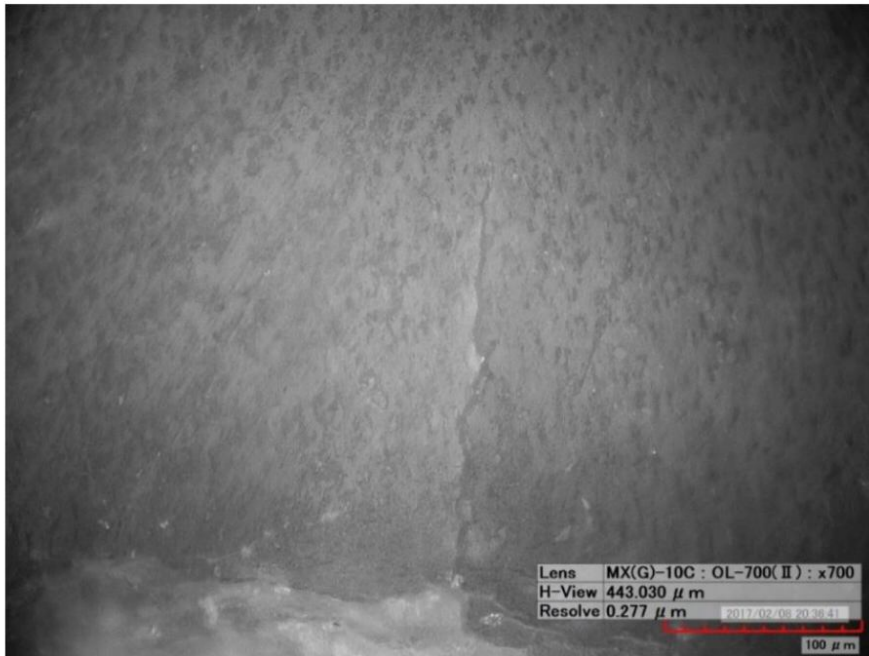
Figure 16: A photograph of a microcrack at 700x magnification
