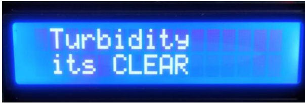
Fig. 11. Displaying the turbidity of the pisciculture system prototype as clear
