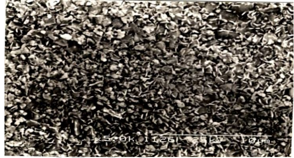
Figure 2b. SEM micrograph of ZnO annealed at a temperature of 600°C for 2 hours.
