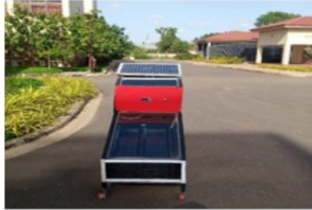
Figure 4b. constructed solar dryer.
