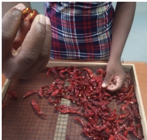
Figure 14: Brittleness of Chilli Pepper in Solar Dryer by 27 th Hour
