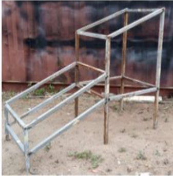
Figure 4a. the frame of the solar dryer
