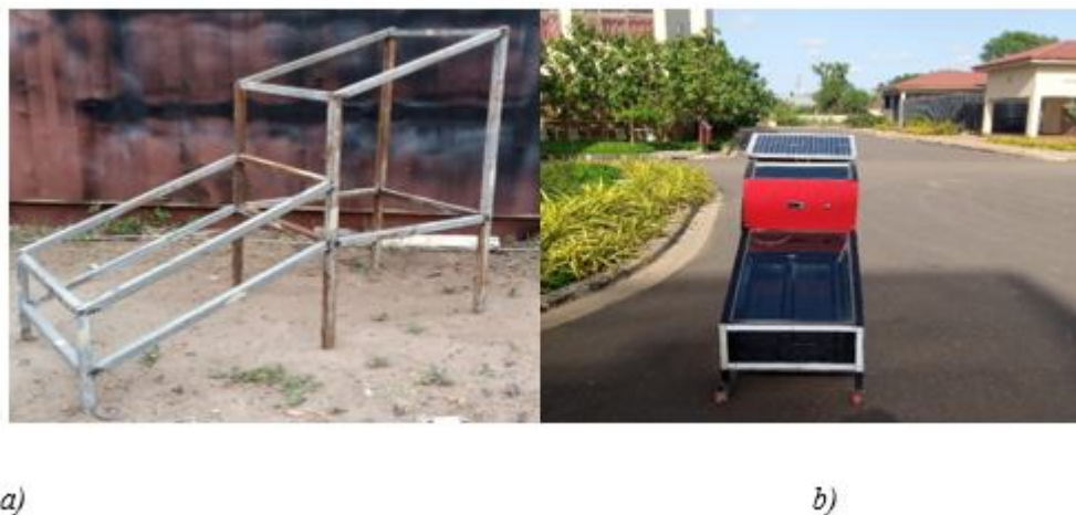
Figure 4: Frame and the finished constructed solar dryer
