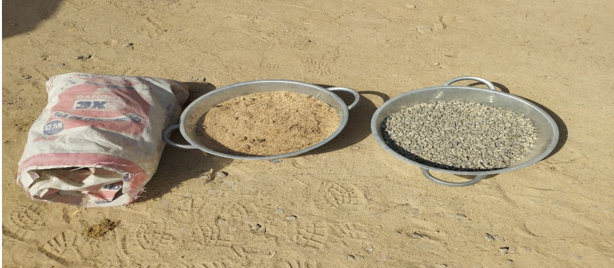
Plate 3. Constituent materials: from left to right: Waste plastic bags, Sand, Granite.
