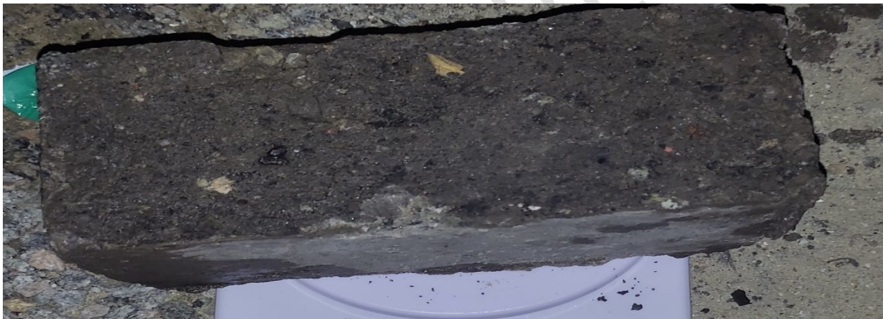
Plate 4. Sample 1, (waste plastic bound paving stone)
