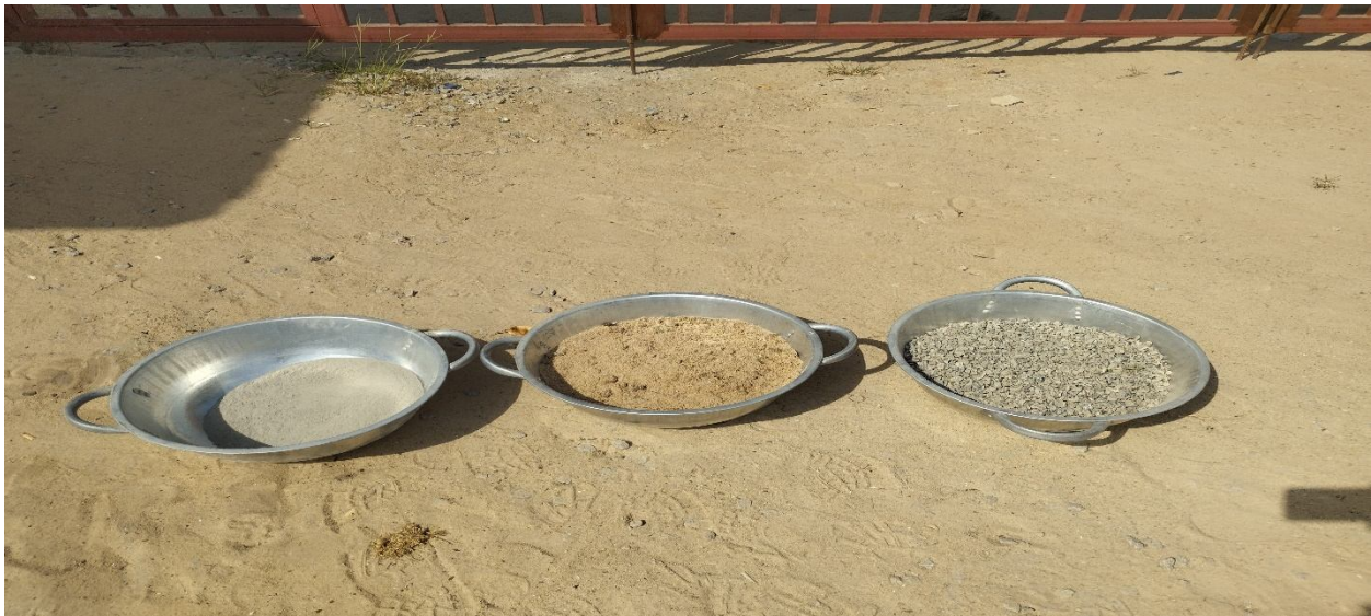
Plate 1. Constituent materials: from left to right: Portland cement, Sand, Granite.
