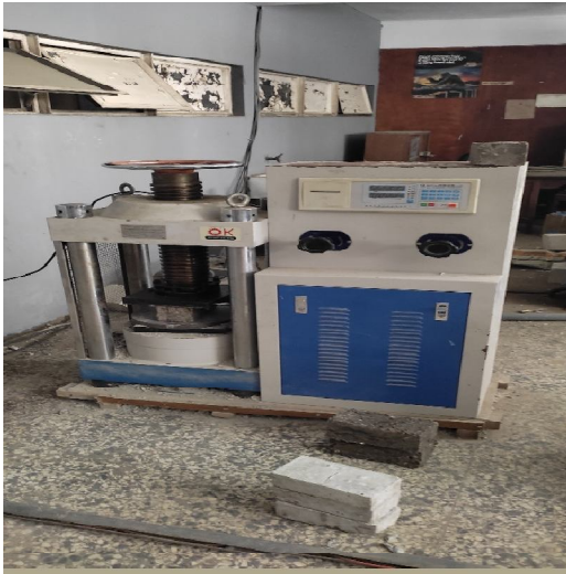
Fig. 6. Crushing of control and sample paving stones.
