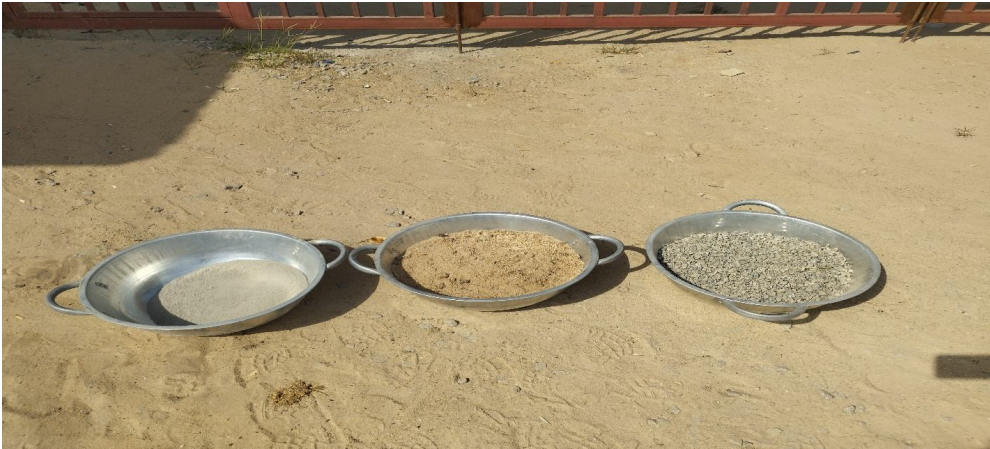
Fig. 2. Constituent materials: from left to right: Portland cement, Sand, Granite.
