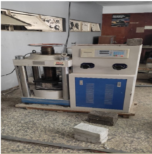
Fig. 6. Crushing of control and sample paving stones.
