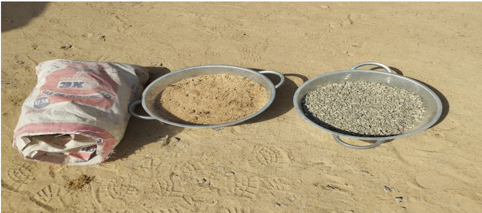
Fig. 4. Constituent materials: from left to right: Waste plastic bags, Sand, Granite.
