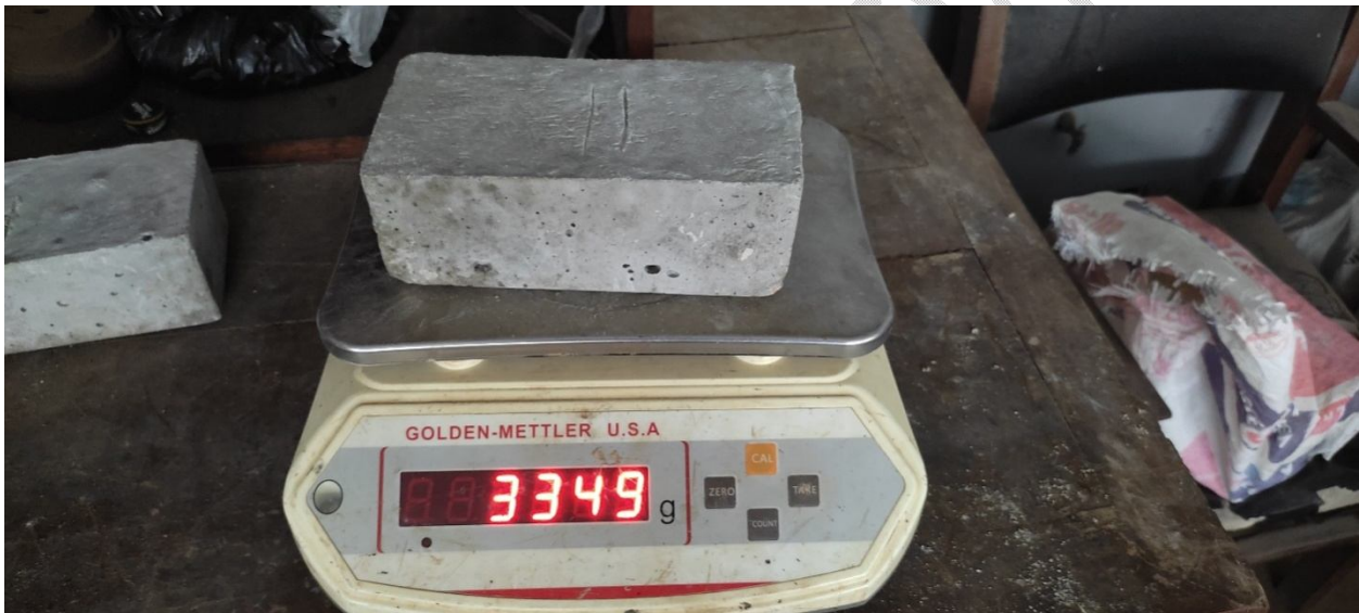
Fig. 3. Control sample 2, (cement-bound paving stone)
