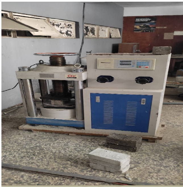
Fig. 6. Crushing of control and sample paving stones.
