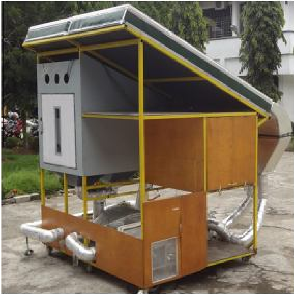
Figure 8. Solar assisted heat pump dryer (SAHPD)
