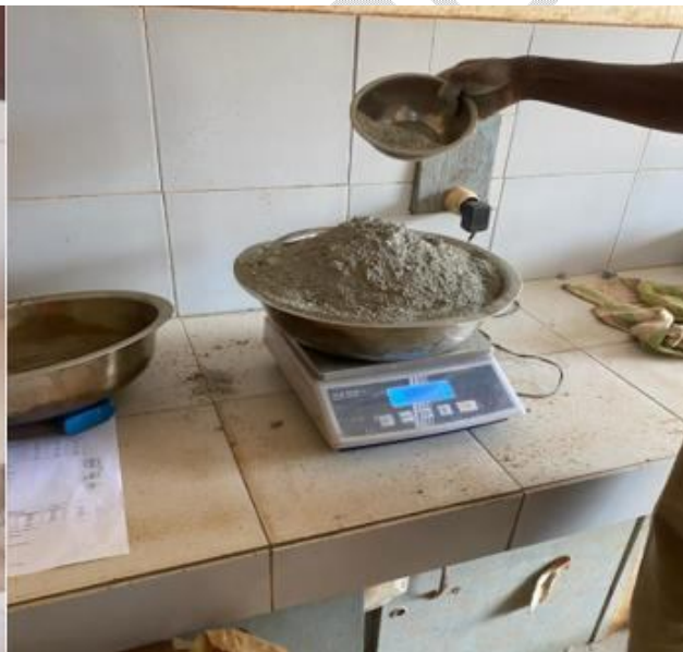
Fig. 4.Measurement of the mass of glass Fig. 5.Measurement of the mass of cement
