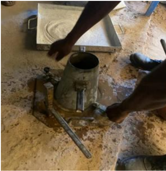
Fig. 8. Photos of sag measurements
