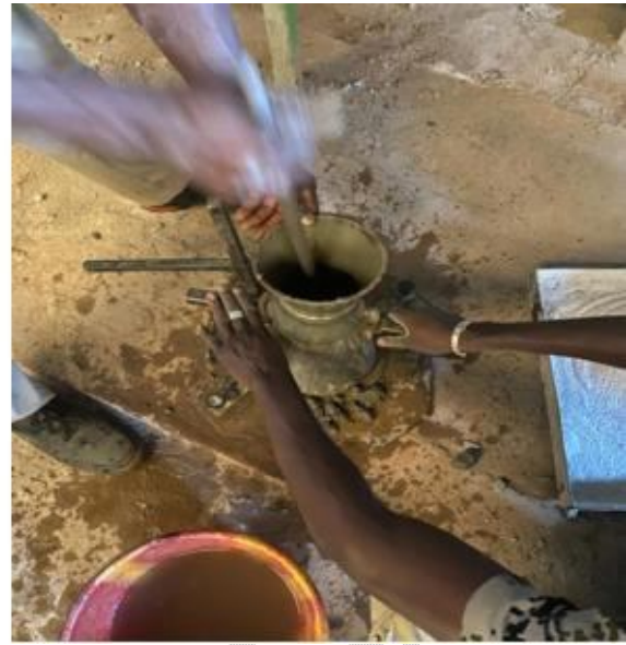
Fig. 8. Photos of sag measurements
