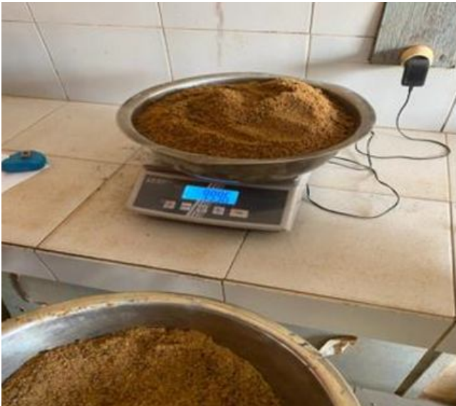
Fig. 2.Measurement of the mass of sand Fig. 3.Measurement of the mass of crushed aggregate
