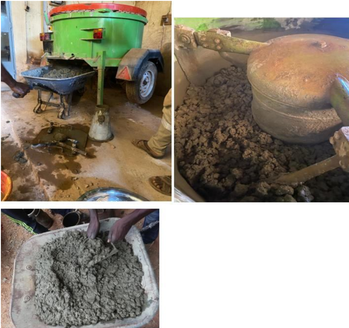
Fig.7.Images of the formed concrete
