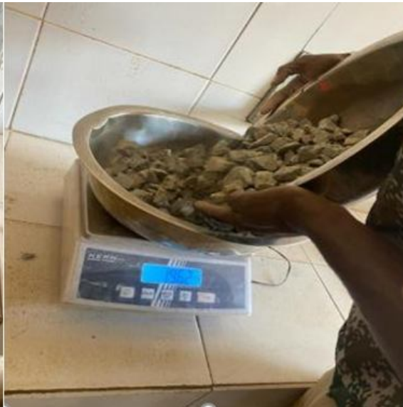
Fig. 2.Measurement of the mass of sand Fig. 3.Measurement of the mass of crushed aggregate
