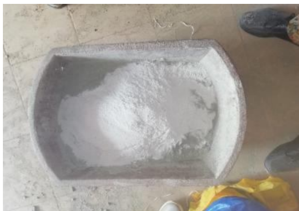
Fig. 6.Mixing glass powder and cement
