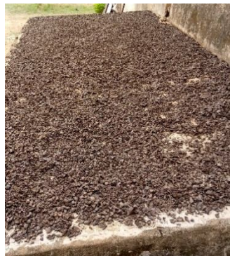
Figure 2 Drying of PKS
