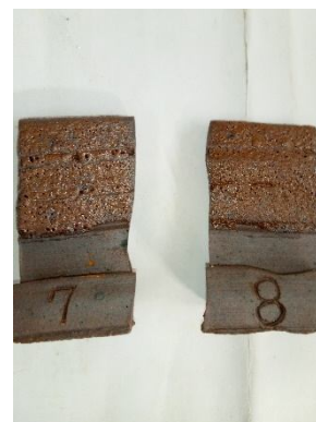
Figure 7 Almost melted tiles.
